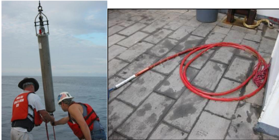
Figure 3-5. OAR-PMEL AUH being deployed, and a towed array on the deck of a ship.
